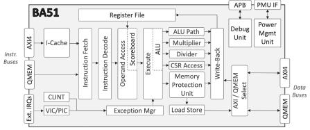
Furthermore, the BA51 supports software and timer interrupts and up to 64 external interrupt lines. It features a remarkably low interrupt response time, which makes the core ideal for real time control applications. The time elapsed from when an external interrupt is asserted until the first instruction in the resolved interrupt handler can be issued is just 4 clock cycles.
