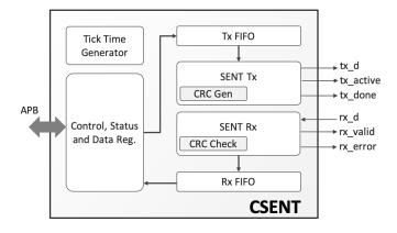
interrupt-based operation. The core allows for Transmitter operation without requiring any external programming or control. The reset values for all its control registers are defined at synthesis time, and at run time the system only needs to write sensor data to the core.
