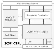
In I2C mode, the I2CSPI-CTRL supports standard, and fast mode with transfer rates of up to 400khz, with both 7-bit and 10-bit addressing. It
